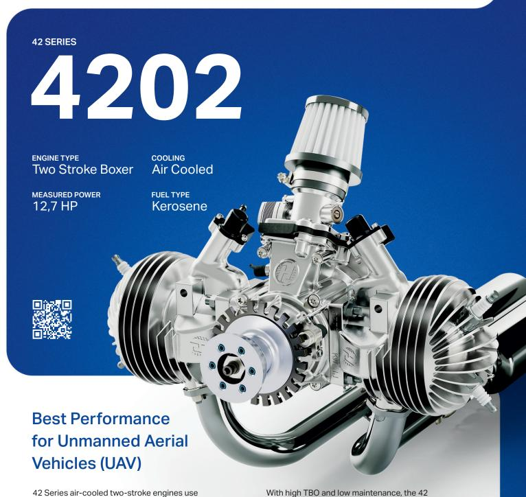
advanced closed-loop control to deliver reliable, lightweight UAV propulsion in tough conditions. The new 4202 Heavy Fuel Engine tops the 15-HP class for power-to-weight and durability, based on the proven 4201 gasoline platform and optimized for JET-A1 after extensive endurance testing.
